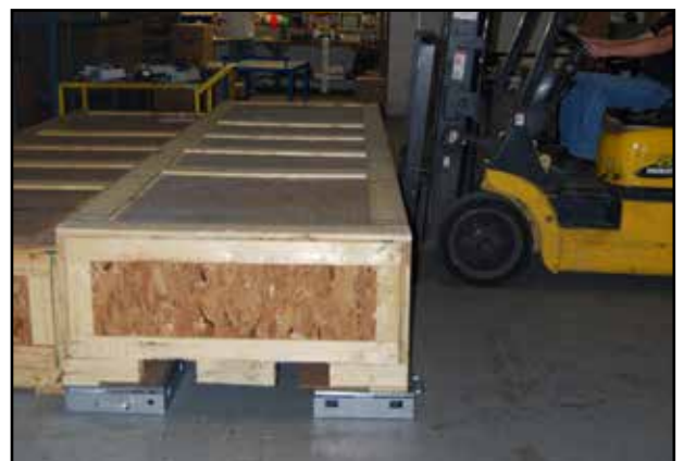
Oversized packages that aren't easily weighed are placed on the SW™ scales.
