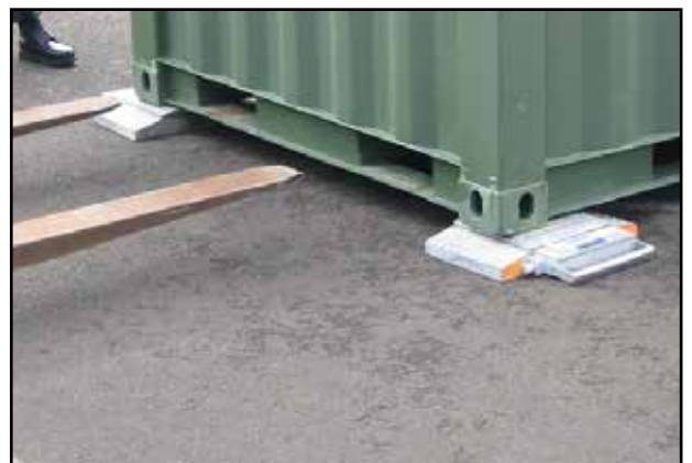
For larger packed containers, Intercomp PT300™ scales can be used for SOLAS Method 1 weight compliance.
